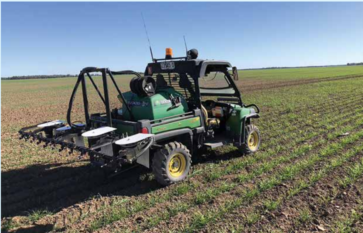
The AutoWeed prototype machine, which uses sensors and deep learning to distinguish weeds from crops (James Cook University).
